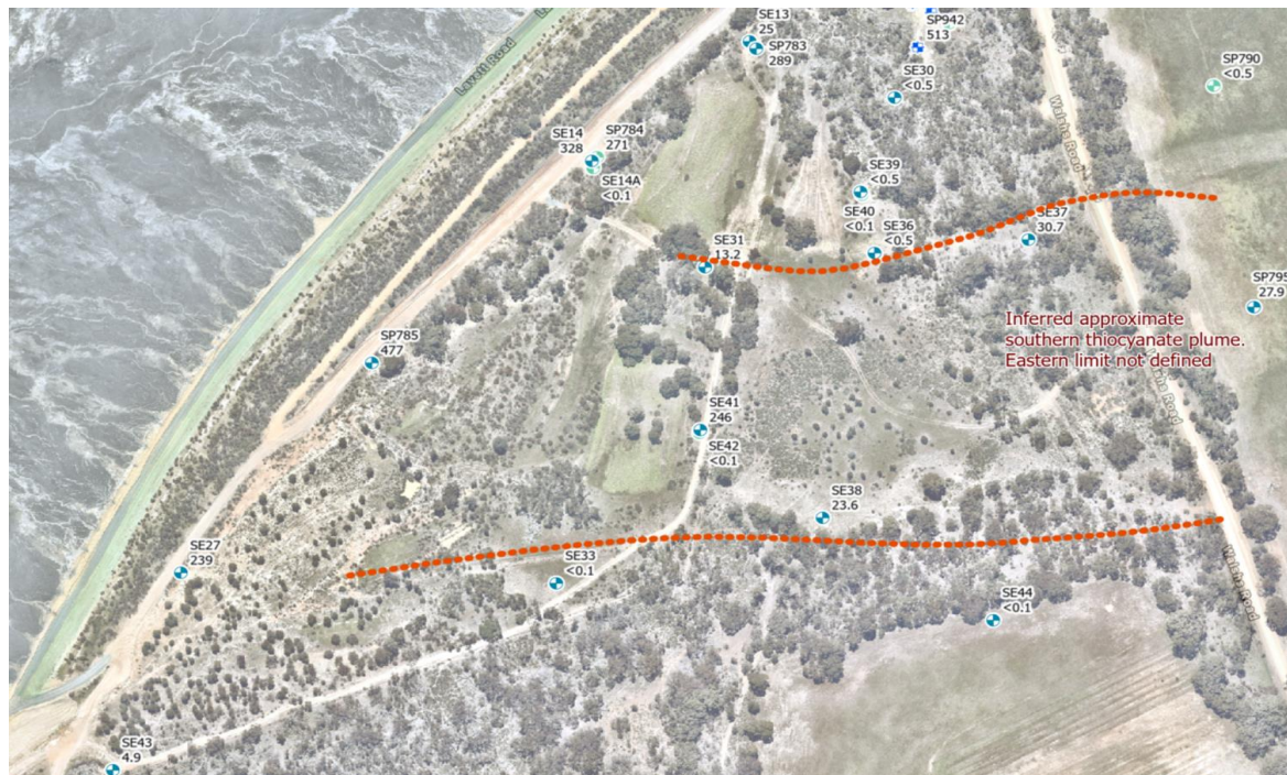
FIGURE 6. HYDRAULIC CONTAINMENT SYSTEM – NEW BORE LOCATIONS
