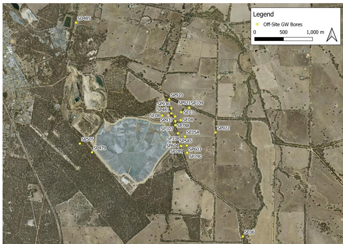
Figure 4 SGM offsite Groundwater monitoring bore locations
