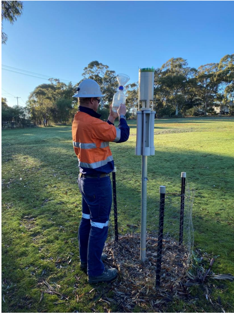
Figure 5 Dust deposition gauge
